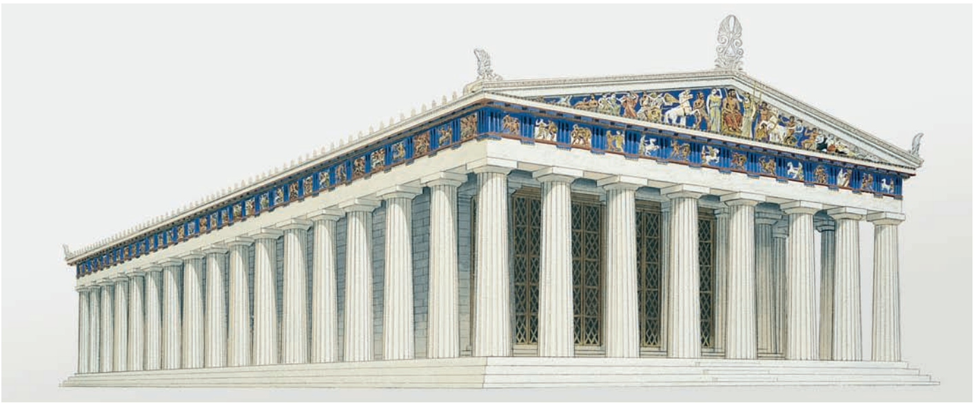
7.18 Reconstruction of the Parthenon, Athens. View of the east façade and south wall. The metopes and pediment sculptures are also reconstructed to show that they were originally painted.
