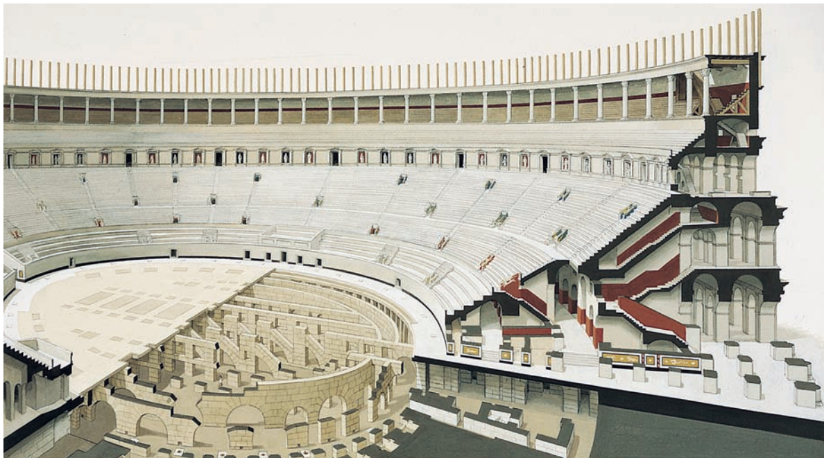
9.13 Reconstructed cutaway section of the Colosseum.
